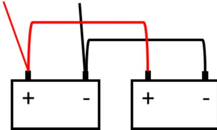
Figure 7: Parallel connection of 12V batteries maintaining a system voltage of 12V
