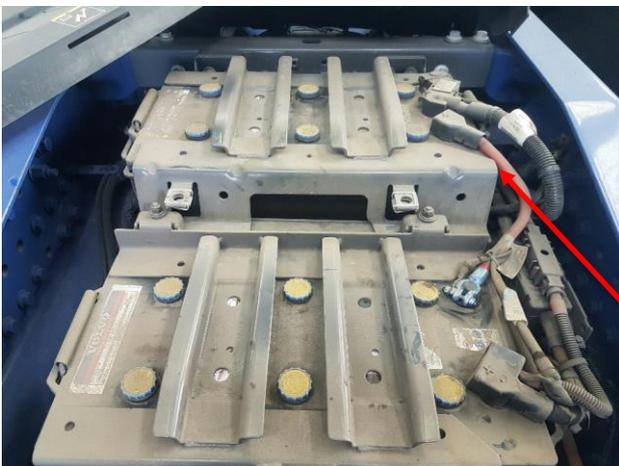
Additionally, this location in the rear overhang between the chassis rails, frees up chassis side rail space and will take mass off the steer axle, but makes jump starting of the unit significantly harder when under a trailer is coupled, unless an auxiliary jump start post is available.
