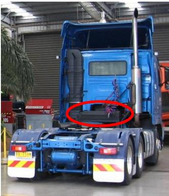
Figure 5: common battery location on a COE prime mover
