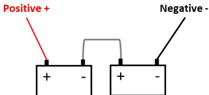
Figure 6: Series connection of 12V batteries producing a system voltage of 24V
