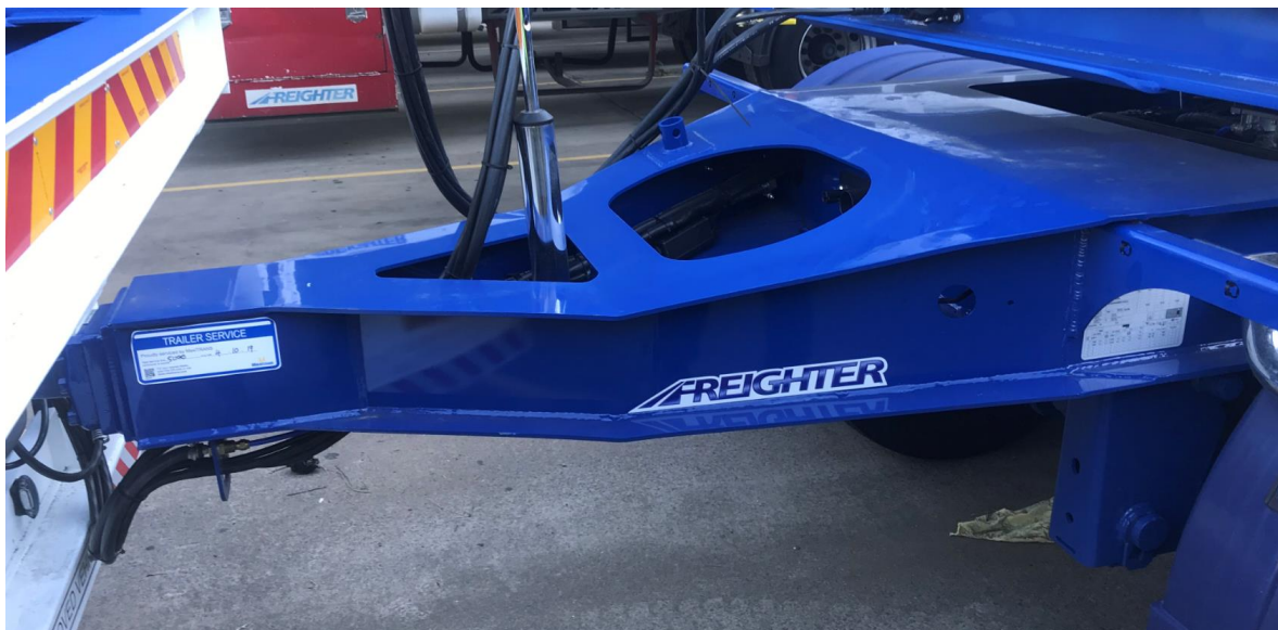
A Rigid Drawbar (tandem) Converter Dolly in a 30 metre PBS A-double Combination
